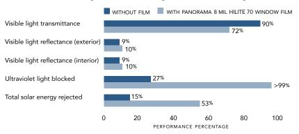
All performance results are based on the film installed on the inside surface of 1/8" (3mm,) 1/4" (6mm,) and 1/8" +1/8" (3mm+3mm) thick, clear glass.
