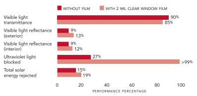
All performance results are based on the film installed on the inside surface of  $1/8^{\ast}$  (3mm),  $1/4^{\ast}$  (6mm), and  $1/8^{\ast}+1/8^{\ast}$  (3mm+3mm) thick, clear glass.
